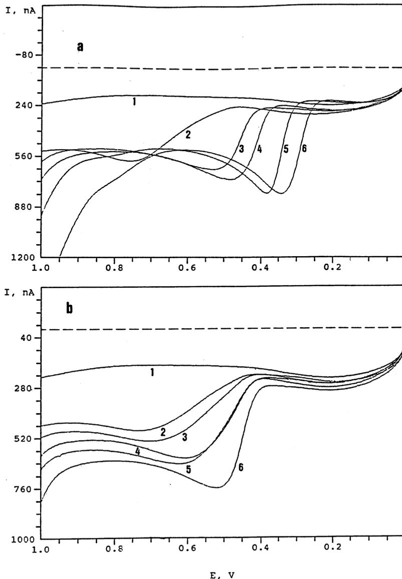
Fig. 5. Voltammograms of a 10 µg ml<sup>-1</sup> olanzapine standard solution, recorded at several pH values (1 = supporting electrolyte; 2 = pH 1.5; 3 = pH 2.5; 4 = pH 3.5; 5 = pH 4.5; 6 = pH 6.5) (a) and several temperature values (1 = supporting electrolyte; 2 = 15°C; 3 = 20°C; 4 = 25°C; 5 = 30°C; 6 = 35°C) (b).
