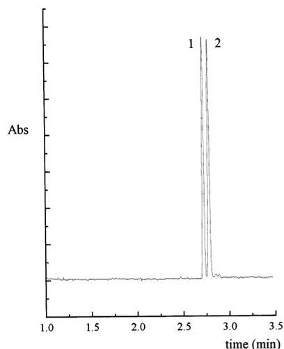
Fig. 3. Capillary zone electropherogram of olanzapine (nominal concentration 25.0  $\mu\text{g ml}^{-1}$ ) obtained from Zyprexa<sup>®</sup> tablets. Peak identification: 1, Olanzapine; 2, IS. Conditions: uncoated fused silica capillary, 43 cm, 23 cm total and effective length, 50  $\mu\text{m}$  i.d. BGE: phosphate buffer (50 mM, pH 3.0). Voltage +15 kV. Detection at 214 nm.
